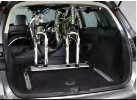
45 | Luggage Bicycle Holder (Rail) L0010AJ007 Easily transport 2 bicycles in the cargo space. (Must remove front wheels.) WGN OBR
